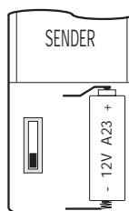
Remove the cover of the battery chamber of the remote control.
